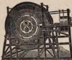
Fig. 245. A churn with worker attachment.
